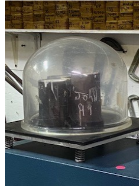
Above Left: Flasks in vacuum to remove bubbles. Above Right: Erleen cleaning silver.
