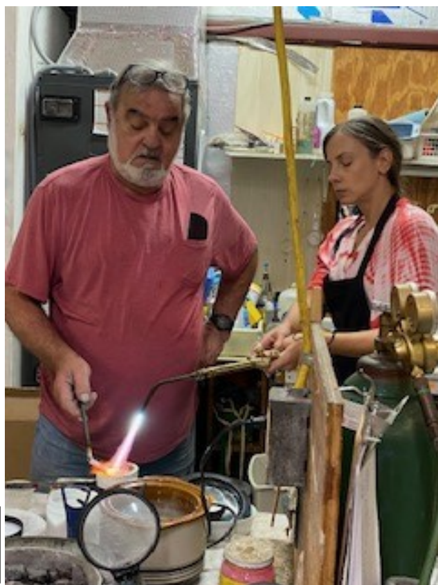
John and Myrriah melting silver using the acetylene torch.
